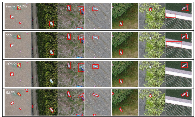
Fig. 11. Visualization results of testing on UAV-BD using well-trained Faster R-CNN, SSD and RRPN. Top to Bottom respectively illustrate the results for Faster R-CNN, SSD, YOLOv2 and RRPN.
